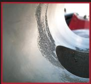
When our customers call to refurbish their equipment, we pick it up at the well site, and then begin the process of refurbishment. One of the first steps is to visually inspect the equipment for possible damage to any of the internal components. In the illustrations to the left, the BOP's in question showed signs of possible chemical attack.
